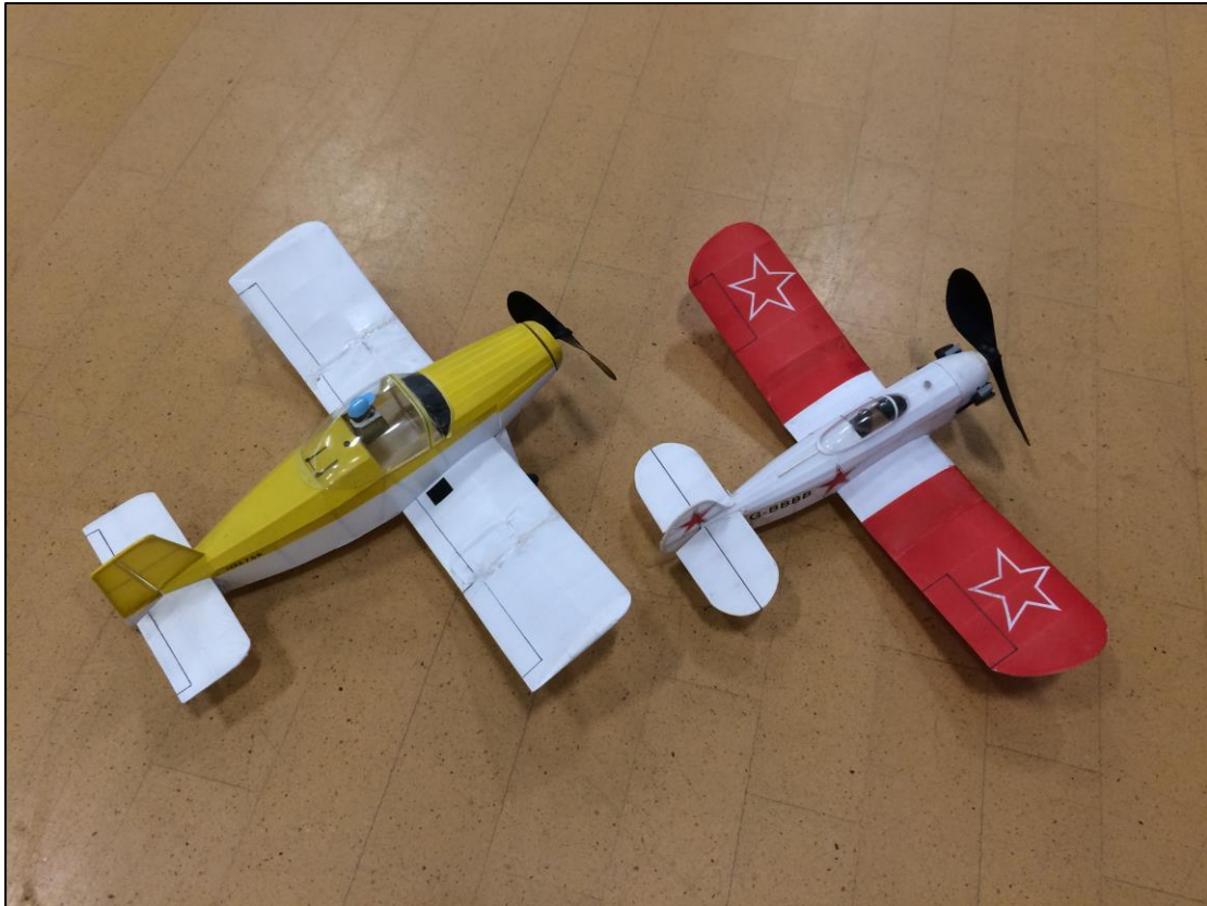
Peter Smart's Thorp T-18 Tiger peanut with his old Taylor Monoplane peanut in USSR 1941 winter colours. The T-18 has had some rather brutal surgery on the outer wing panels because, as built, it was laterally unstable.
