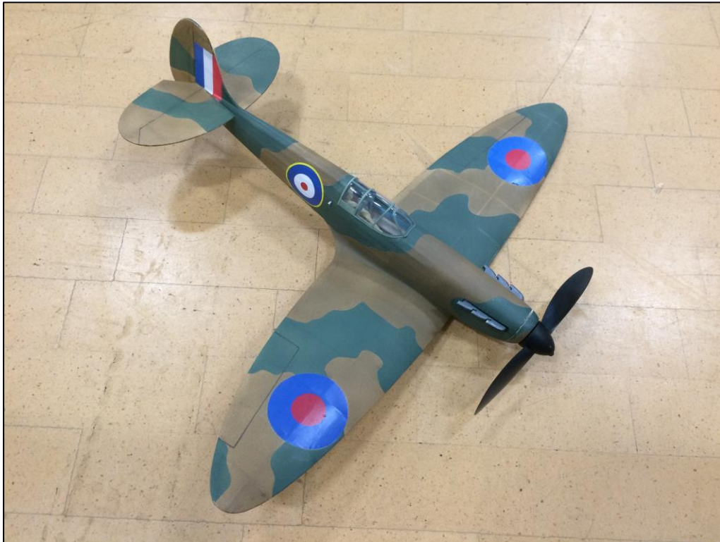
Mick Langford's VMC Spitfire, 37 grams powered by 4 strands of 88 thou rubber 15 1/4" long. Has flown two circles, trimming is ongoing. A bit tricky to launch.
