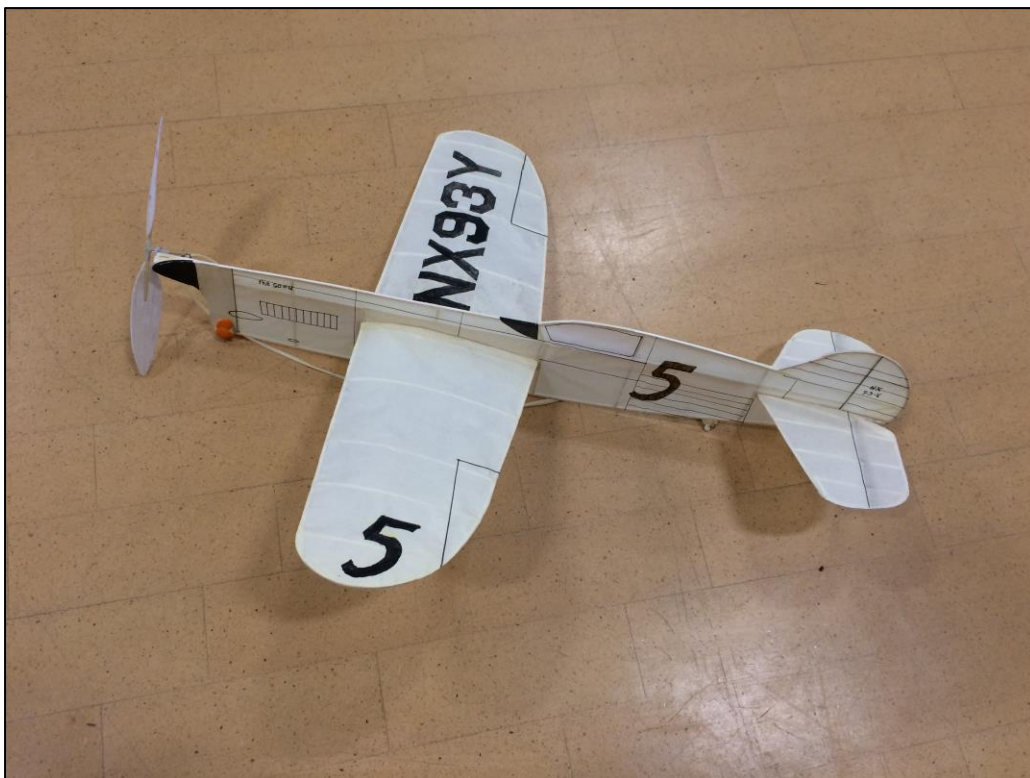
Dave King's own design Art Chester Goon No Cal, 16" span weighs 7.5 grams empty, has only done about 30 seconds so far but shows promise.
